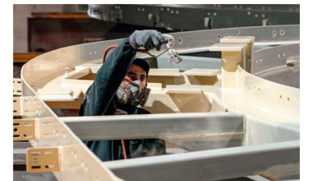
Airless spraying requires excellent skills from the painter in order to eliminate overspray or the so-called orange skin, with proper coat thickness maintained.
